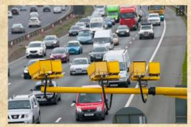
The first camera type is still used today and is named the Gatso after Dutch rally-driving inventor Maurice Gatsonides. The Gatso is a type of fixed speed camera which means that it records the speed at which a car passes at a particular location.
