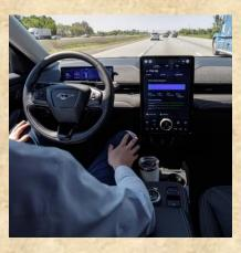
The "hands-off, eyes-on" technology, level two on the automation scale, monitors road markings, speed signs and traffic conditions to control steering, acceleration, braking and lane positioning. It is also designed to maintain 'safe and consistent' distances to vehicles ahead - right down to a complete halt in traffic jams. The technology features a sophisticated infrared camera which continually checks driver attentiveness for safety and confidence.
